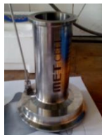
Figure 2. Laboratory model of a flat membrane filtration cell
