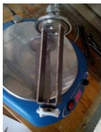
Figure 2. Laboratory model of a flat membrane filtration cell
